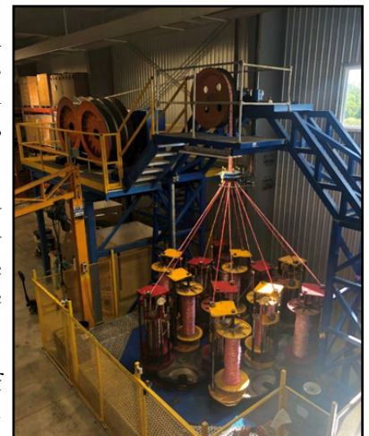
Atlantic Braids rope producing machine.
