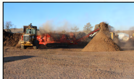
Rough mulch being regraded and screened
